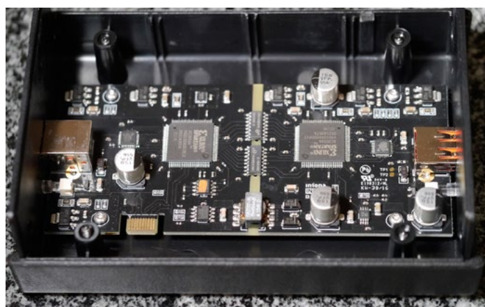
Two discrete PCB joined only by digital isolators to "cut the cord" between computer and DAC. Even visually the "dual everything" concept makes sense.
