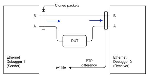
Ethernet Debugger 1 is the sender, Ethernet Debugger 2 is the receiver. The sender generates packets that get sent out of port A and B at the same time. DUT is expected to propagate the packet unchanged to the receiver. The receiver measures the difference in arrival time between port A and B.
